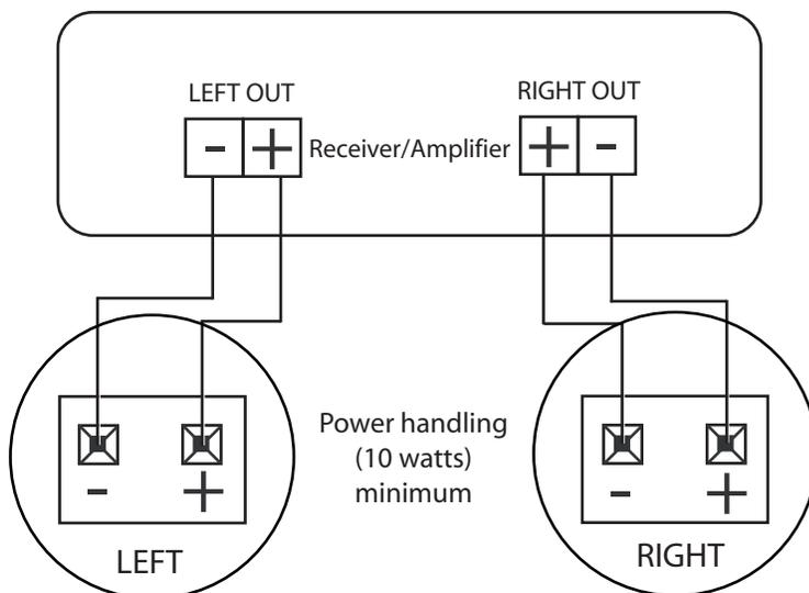
Note: Speaker terminals have corresponding (+) and (-) terminals. It is important to connect both speakers in phase. Out of phase will result in thin sound and weak bass.
